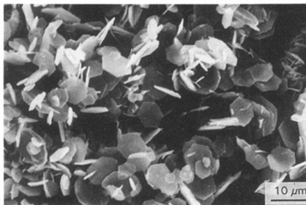
Figure 5 Scanning electron micrograph of strontium hexaferrite synthesized hydrothermally at 220 °C for 5 h using an \text{OH}^-/\text{NO}_3^- molar ratio of 6.
